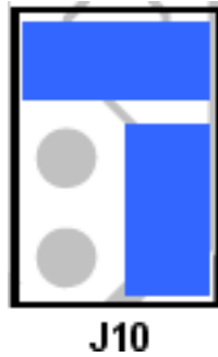
Figure 7 J10 Jumper settings for Current output
