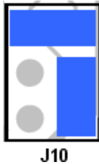
Figure 7 J10 Jumper settings for Current output
